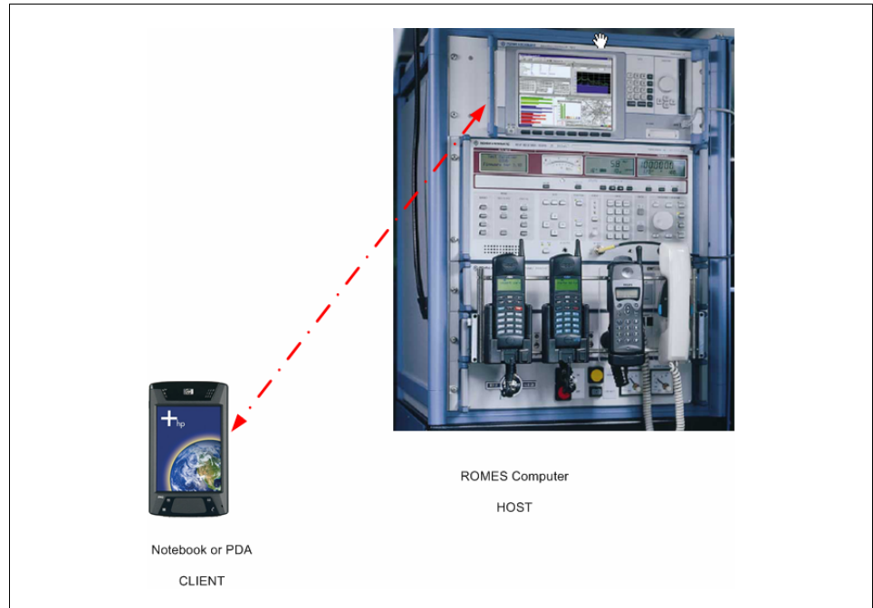
Figure 1: Principle setup of a remote controlled ROMES system
